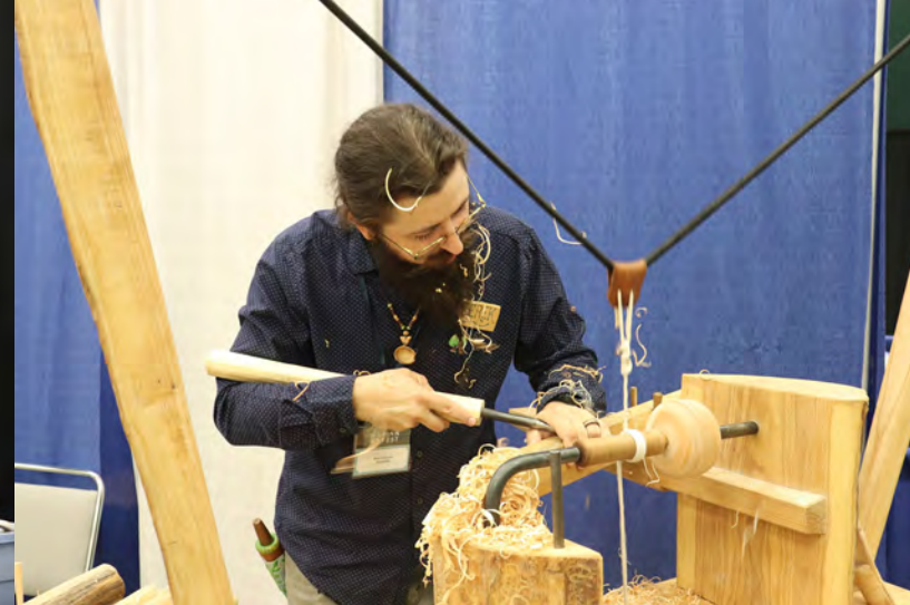
Derek Brabender demonstrates pole lathe turning in action. Photo credit: Jason Schroeder.
